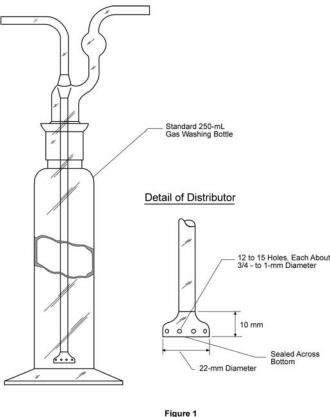
Gas Washing Bottle with Perforated Disk Gas Distributor
